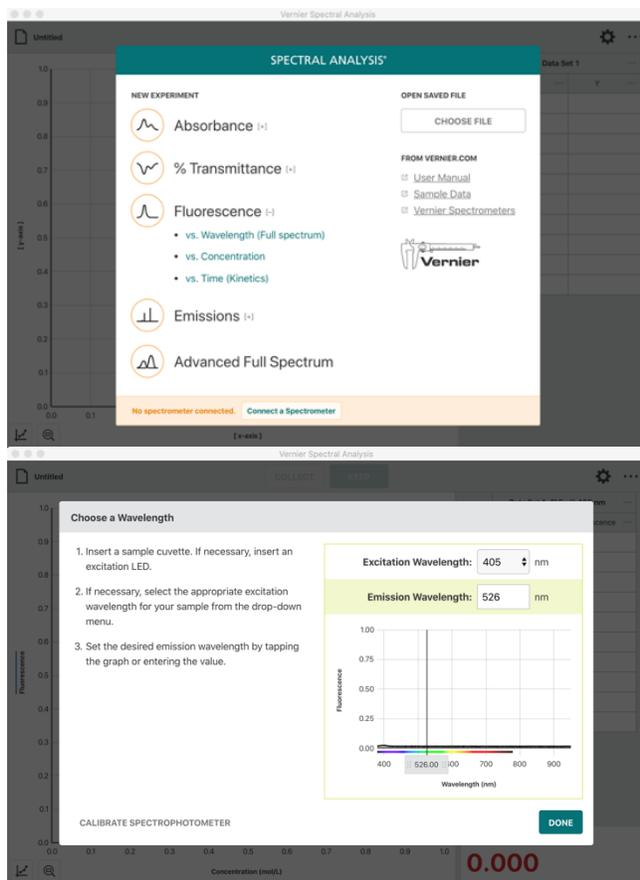
confirm excitation wavelength, then press “Calibrate”. A new window will appear. With your blank placed in the instrument, select “Finish Calibration”. Once complete, your spectrometer should be “zeroed”. This is indicated by a reading of approximately 0.000 in red in the bottom corner of the window.
