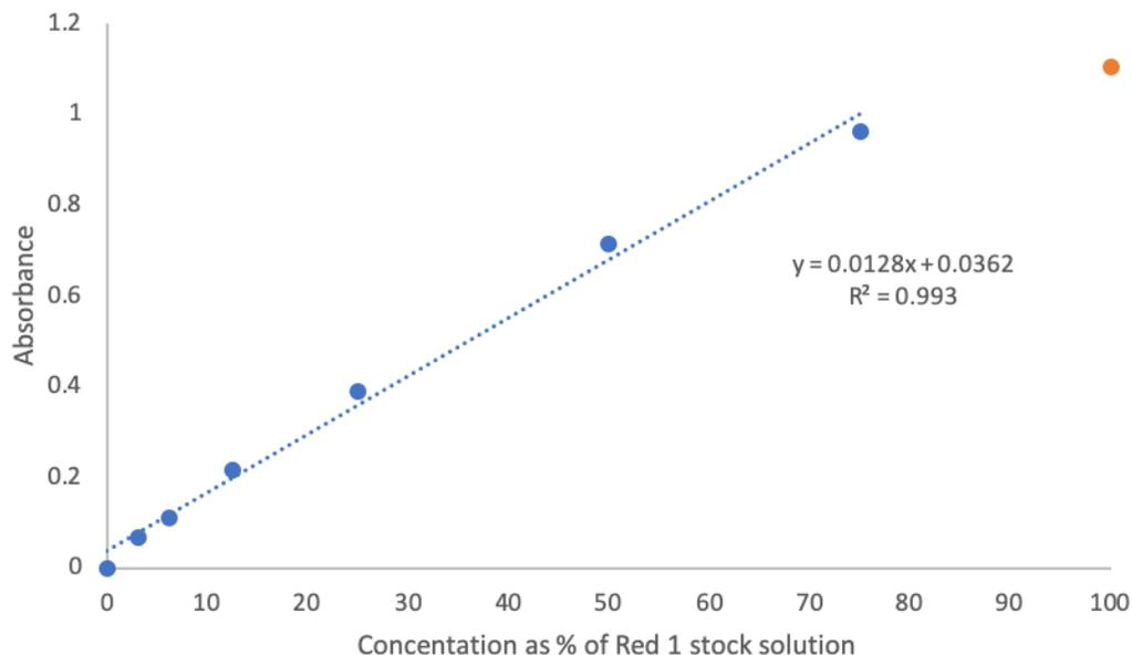
There is rollover at absorbance values around 0.8-0.9 and is much more pronounced when the absorbance is above 1. This is probably due to stray light and a non-linear signal correlation when low amounts of radiation traverse the photoresistor.
