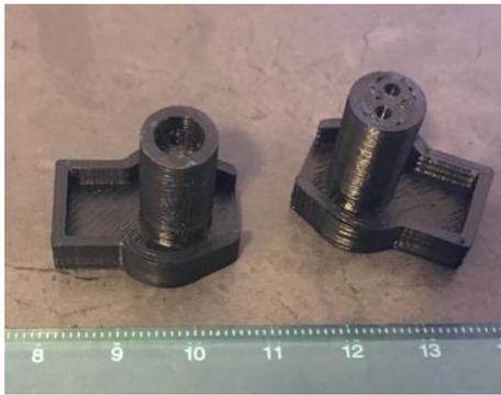
End caps for LED and photoresistor (this is the print file from Porter)
