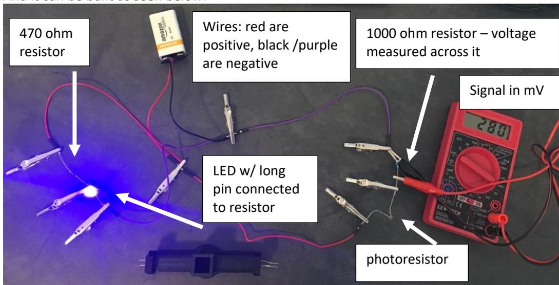
You can see the 470 ohm resistor on the far left acting as a ballast resistor to limit current through the LED so it doesn't burn out. The LED is attached to the resistor on the long pin as that identifies the positive end of the LED. For the photoresistor, order of the resistors or orientation for connection do not matter.
